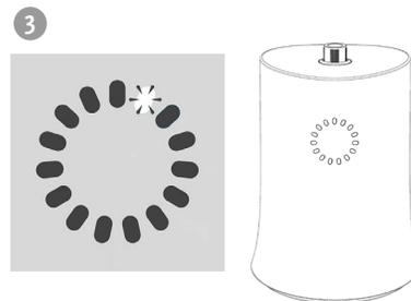
Beginning of solid to liquid phase change is detected by unit.
