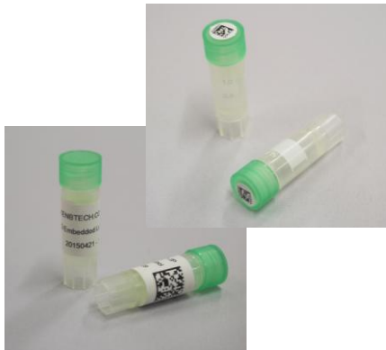
RFID tag embedded in ultra-low temperature resistant label
